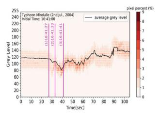
**Fig. 2** Temporal variation of average grey level in Ai-Yu-Zi creek for Typhoon Mindulle. The first 25 s is noise before the debris flow arrives. The black line is the average grey level. Darker color indicates a larger proportion of pixels at that grey level. Pink lines indicate the time locations for images in Fig. 1
