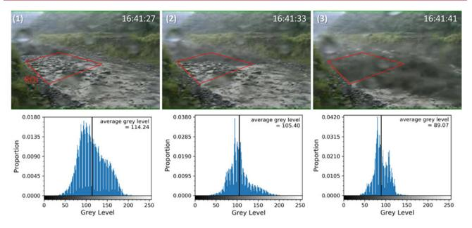
**Fig. 1** Grey-level distributions from video of the Typhoon Mindulle debris flow. 'Proportion' denotes the ratio of the number of pixels of a given grey level to total number of pixels in the ROI (region of interest). Next to the grey-level axis, the corresponding brightness is plotted as a grey-level bar. The vertical line indicates the position of the average grey level for that image. (1) Debris flow just entering ROI
