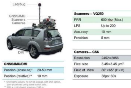
Figure 4. Sensor specification for this research
