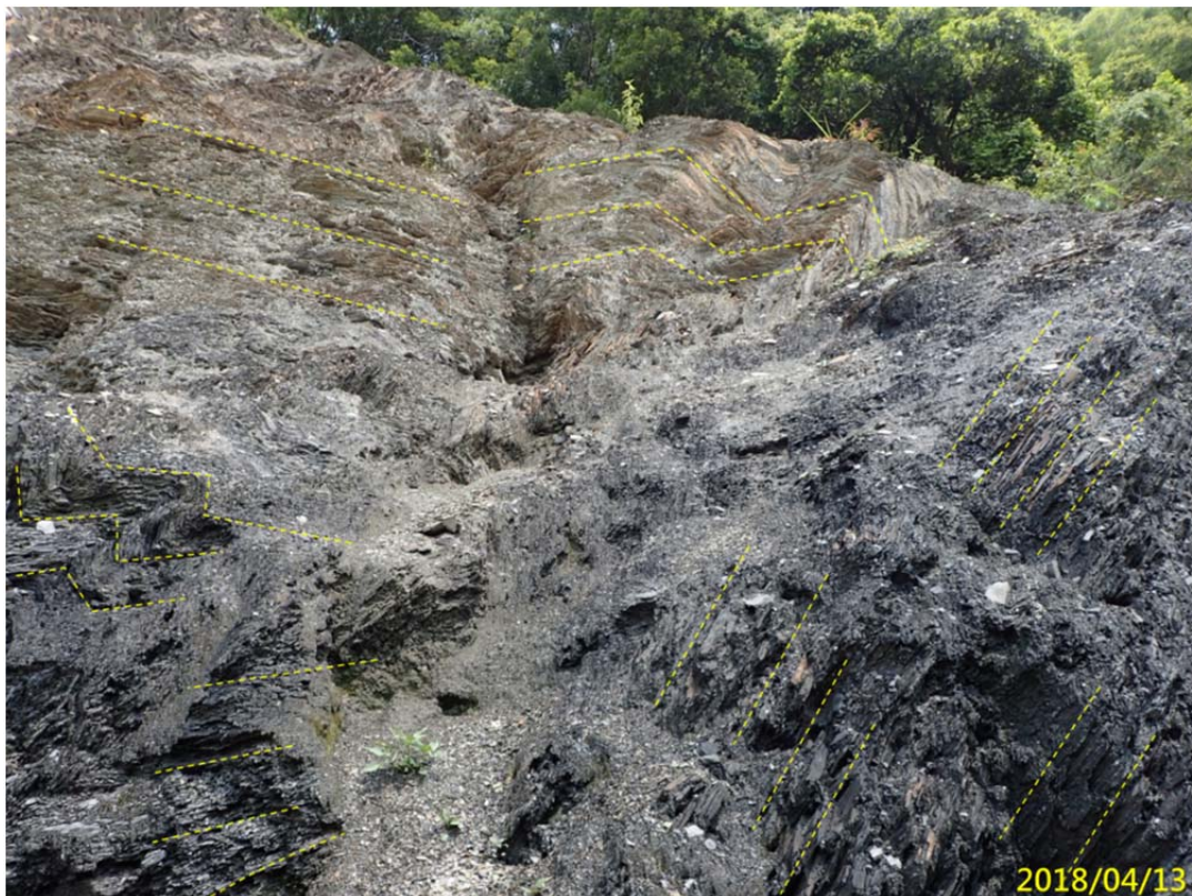
圖 3-15、廬山聚落下邊坡裸坡區，可見灰黑色剪裂帶出露，劈理面呈波浪般的變形 Fig. 3.15 Gray-black shear zone outcrops and the cleavage plane deforms like wave at the lower uncovered slope area of Lushan settlement
