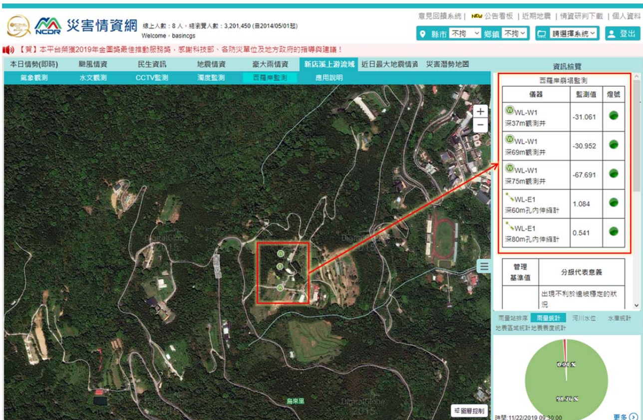
圖 7-6、NCDR 災害情資網介接本計畫西羅岸調查區觀測資料及警戒管理燈號情形 Fig. 7.6 Providing the interface service of observation data and early warning light of Hisloan area to NCDR
