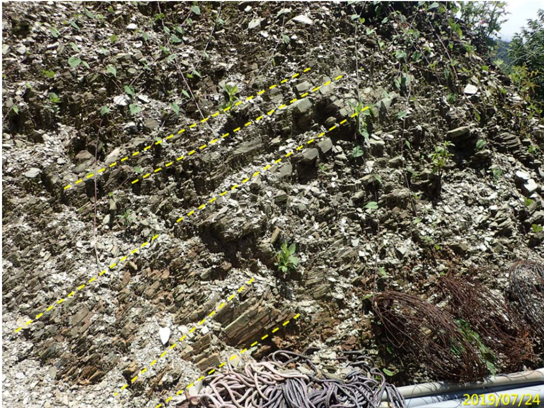
圖 3-18、廬山聚落附近露頭。劈理朝西傾斜，與坡趾朝東傾斜之劈理傾向相反 Fig. 3.18 Cleavage outcrop at Lushan settlement toward west to incline, which is opposite to cleavage east to incline at the toe of slope
