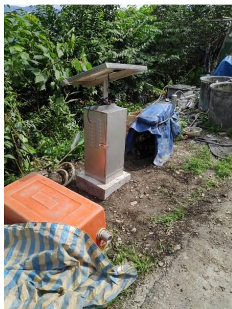
Figure 4.1.2-6 In-situ installation of TDR deformation monitoring cable in 108-D007-2T
