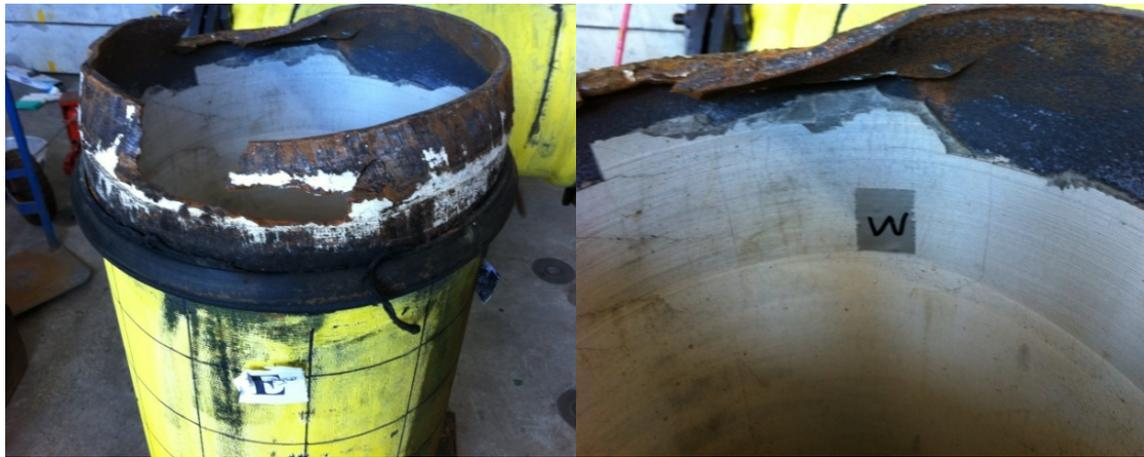
(a)承口端鑄鐵彎曲破壞
