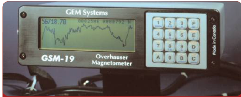
Overhauser (GSM-19W) Walking Magnetometer console. Can also be configured with additional sensor for gradiometer (simultaneous) readings.
