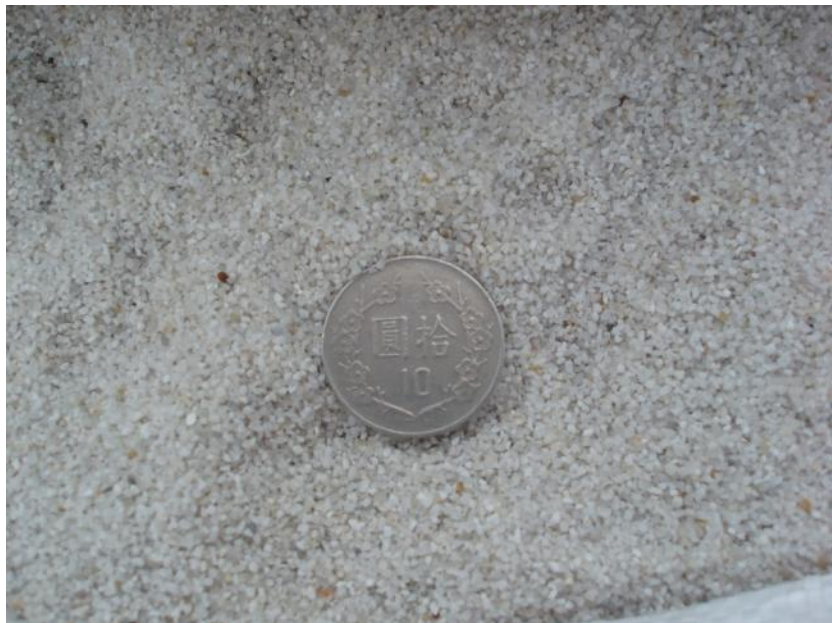
(b) 試驗細砂( D_{50}=0.10\text{cm} )
