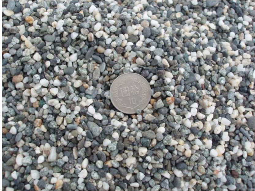
(a) 試驗粗砂( D_{50}=0.32\text{cm} )
