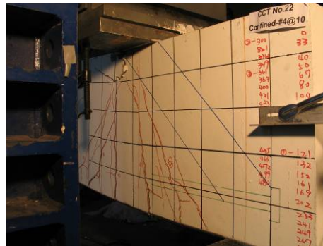
(n) Failure Point
