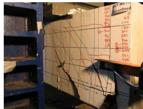
(k) Failure Point
