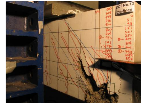
(l) Failure Point
