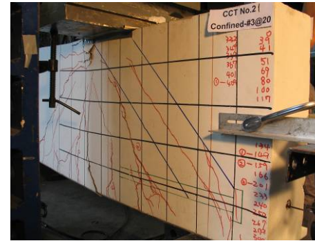
(k) Failure Point
