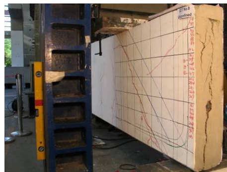
(j) Failure Point
