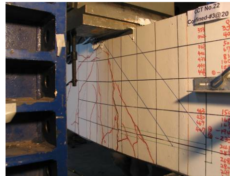
(n) Failure Point
