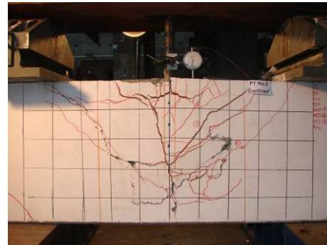
(g) Failure Point
