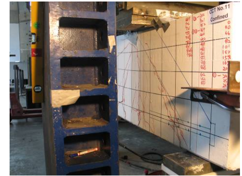
(l) Failure Point
