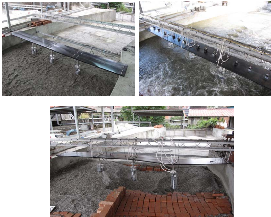
Fig. 2: Photos of the bridge test site and the test specimen, (a) before scouring test, (b) under scouring test, (c) after scouring test.
